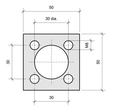
PLATE REFERENCE: **PL00 SQ** WELD TO BEARING: **4.053** USE WITH STEEL CHANNEL: **EC053**
